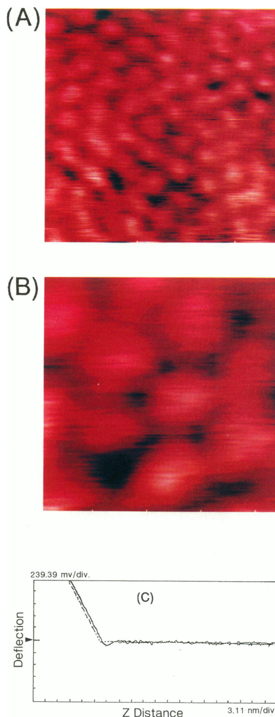
FIGURE 1 (A) Unfiltered AFM image of a regular array of ferritin molecules bound to a PBLH layer on a silicon wafer. The imaging was carried out in pure water using a fluid cell. Image area is 125 \times 125 nm 2 . (B) Higher magnification AFM image showing a hexagonal packing of ferritin molecules. Image area is 45 \times 45 nm 2 . (C) Force curve for Fig. 1 A. Cantilever deflection in millivolts ( ordinate ) versus distance between stylus and sample in nanometers ( abscissa ). The two curves are for approach ( dashed line ) and for withdrawal ( solid line ) of the stylus from the sample. Arrowhead ( \blacktriangleright ) indicates the operation point. It was estimated from this curve that the force applied was 10^{-10} N \sim 10^{-11} N.
